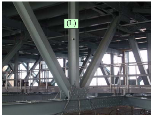
(a). Accelerometer placement on stiffening truss
